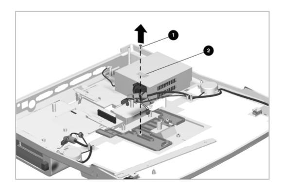
Figure 6-33. Removing the Puller Plate Spring
